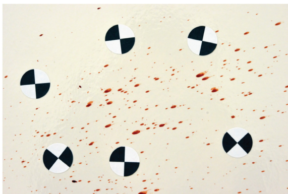
Figure 2 Photograph used in the analysis with reference markers well distributed around a cluster of bloodstains.
